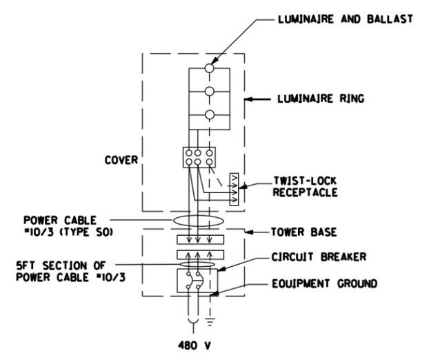
**WIRING ARRANGEMENT AT TOWER LOCATIONS**
