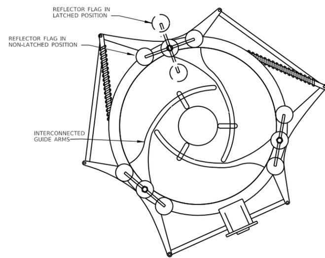
LUMINAIRE RING ASSEMBLY - TOP VIEW
