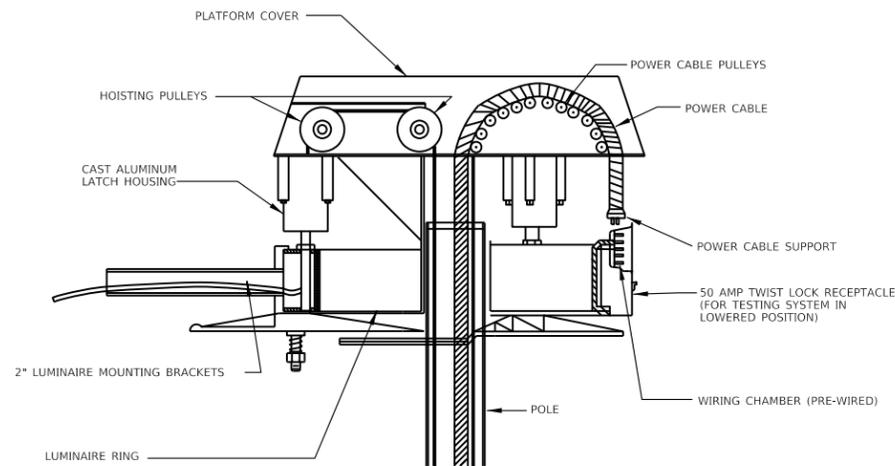
HEADFRAME & LUMINAIRE RING DETAILS - ROTARY LATCHING TYPE
