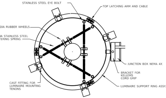
HEADFRAME & LUMINAIRE RING DETAILS - LATERAL LATCHING TYPE
