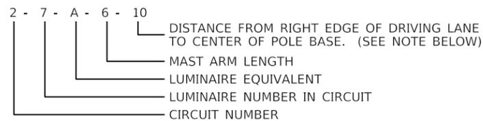
NOTE: IF NO SETBACK DIMENSION IS INDICATED, THE MAST ARM LENGTH DENOTES THE DISTANCE FROM THE RIGHT EDGE OF PAVEMENT TO CENTER OF POLE BASE.
